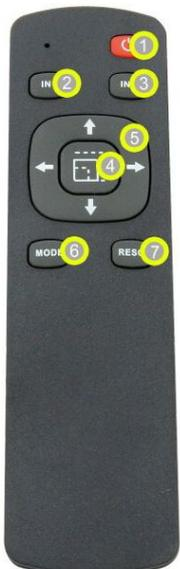
1. **POWER:** Press this button to power on the matrix or set it to standby mode.
