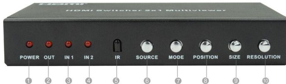
**1.POWER LED:** This red LED illuminates when the device is connected with power supply.
